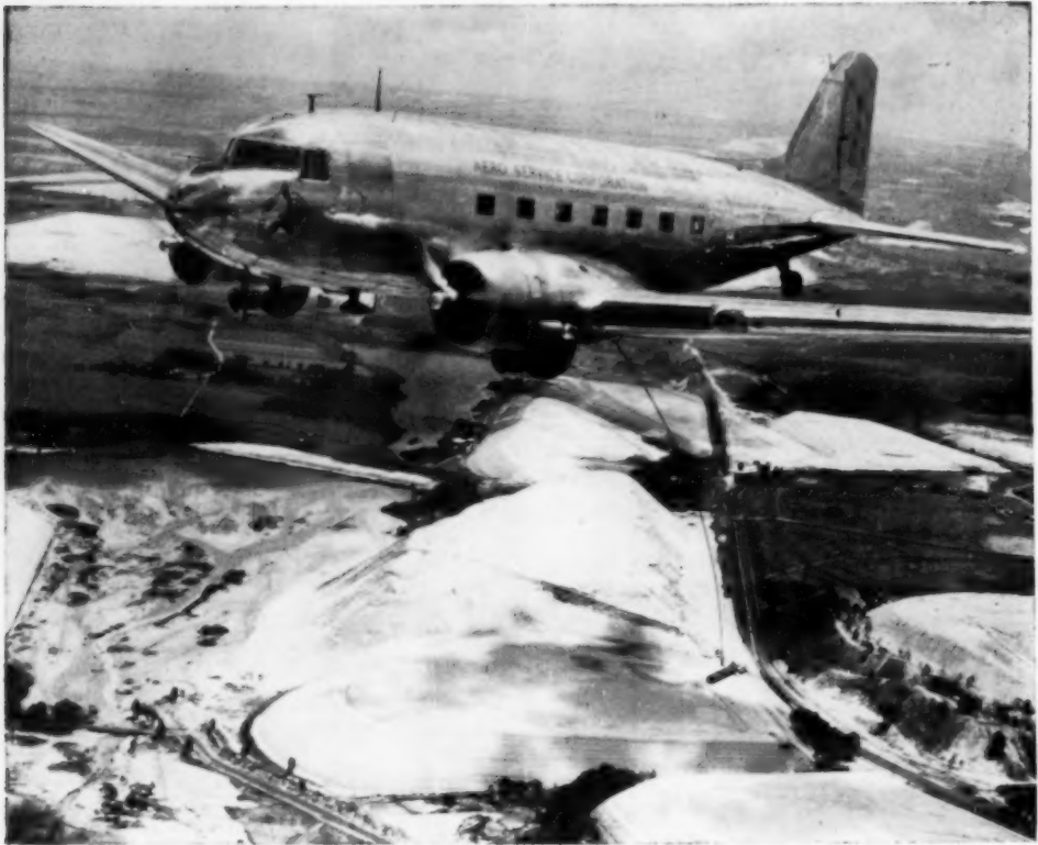
The airborne magnetometer is seen trailing below the survey plane, a specially outfitted Douglas transport, which is pictured here over the waste sludge piles of gold mines in the Union of South Africa.
